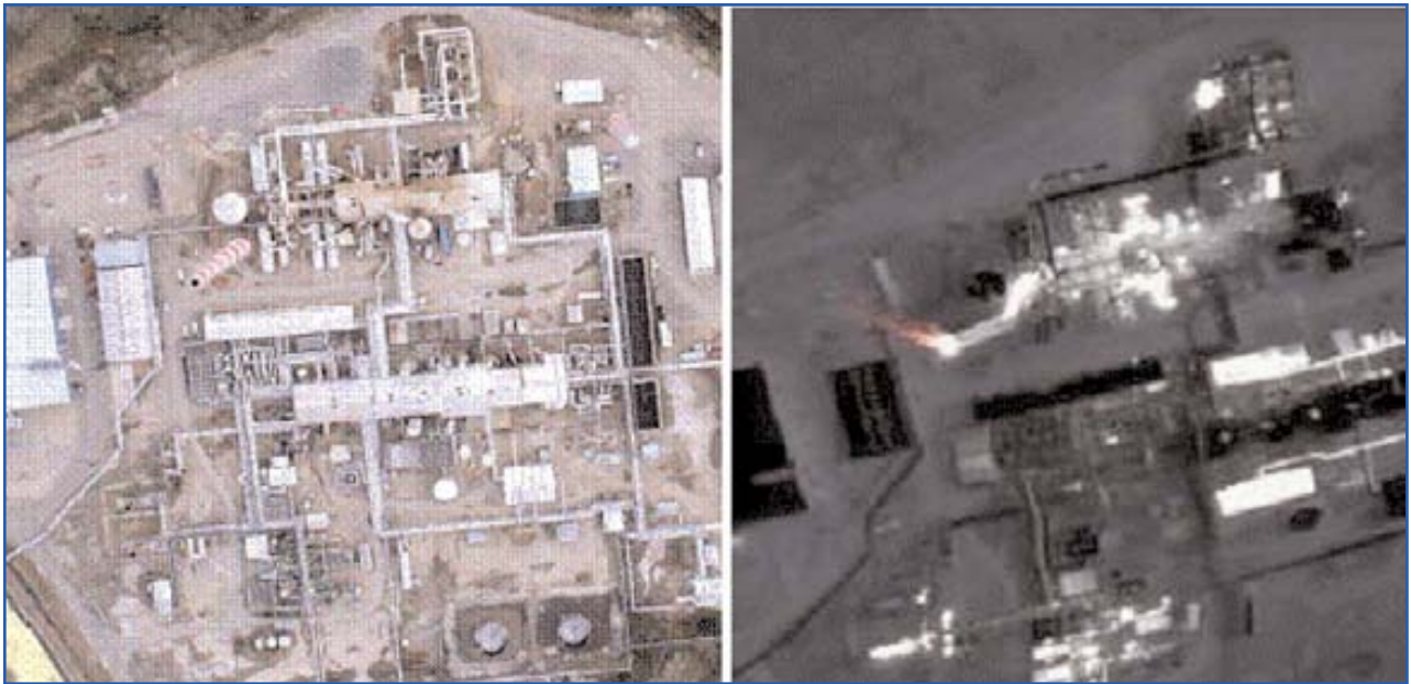
Two images of a sulphur recovery plant emitting gases through its chimney. The gases are invisible in the optical range, but are identifiable in the thermal interval
